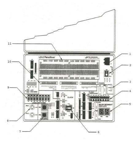
FIGURE 1. Location and description of operating controls.
