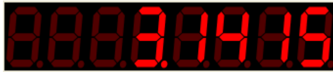
Figure 8. Picture of eight seven-segment displays in one package showing the number 3.1415.
