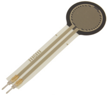
Figure 21. Picture of a force-sensing resistor.
