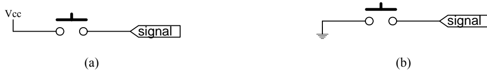
Figure 13. (a) Incorrect circuit that only results in a logic 1 signal when the button is pressed; (b) incorrect circuit that only results in a logic 0 signal when the button is pressed.
