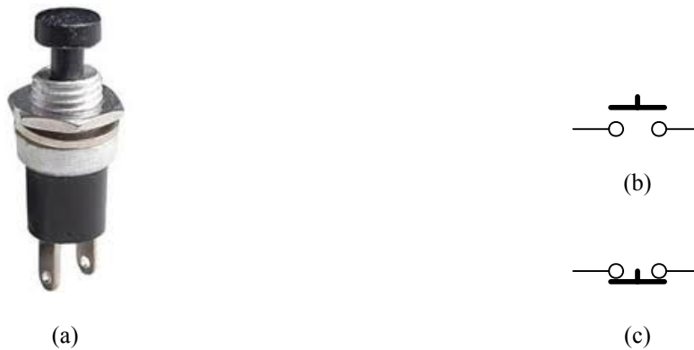
Figure 12. Push button: (a) picture; (b) schematic diagram of a normally-opened push button; (c) schematic diagram of a normally-closed push button.
