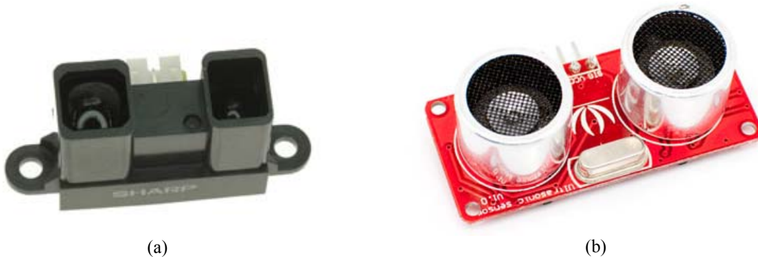
Figure 25. (a) Picture of an infrared red proximity sensor; (b) picture of an ultrasonic distance sensor.
