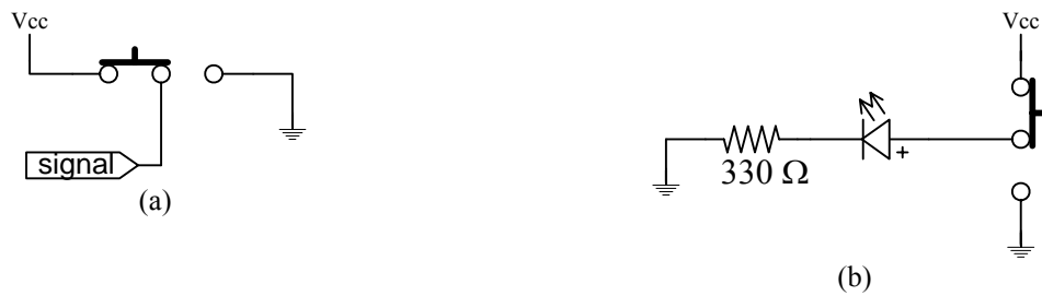
Figure 11. (a) A typical connection for a slider switch; (b) connecting the switch to a LED.
